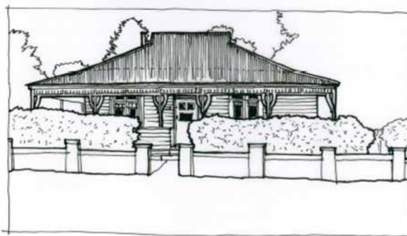
Part D - Figure 11: Farmhouse cottage c. 1910 with verandah roof 'broken back' to the main roof (change of roof pitch), and decorative verandah detailing including timber frieze with spindles and decorative posts and brackets. Brick fence is uncharacteristic; a timber picket fence would be more appropriate to the period.
